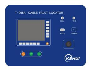
Combines Time Domain Reflectometer (TDR), Impulse Current Method (ICM) and Secondary Impulse method (SIM) for fault detection, T-905A Power Cable Fault Locator is designed to locate all kinds of power cable faults, such as open circuit, short circuit, low insulation, high insulation and flashover faults for electric power industries.
